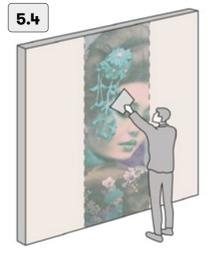
then, level the fiber glass roll with a plastic spatula avoiding any damage to the wallpaper face surface. In case there is not enough glue to perfectly apply the wallpaper rolls to the wall, add further glue on the face surface until the roll is completely covered.
